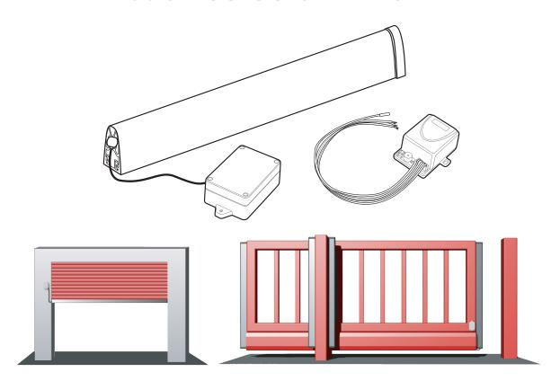
The safety edge system can be installed in the automation gate openers electric window openers, etc moving parts, could prevent the dangers of moving parts, make the whole system stop or stop and rebound to open when it detected a person or object touching it. The elastic material absorbs the impact characteristics and reduces the collision between people and objects.
