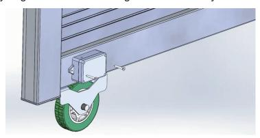
Step 2. Fixed the safety edge on the gate and locked by the screws.
